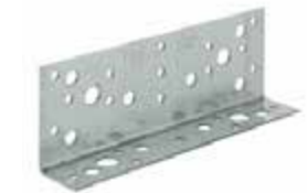
Angled Bracket - BNV33 Manufacturer: strongtie.lv Declarations of Performance : UK-DoP-e06/0106; Technical approvals : ETA-06/0106; Material Steel quality: S250GD + Z275 according to DIN EN10346 Corrosion protection: 275 g / m galvanized on both sides 20mm Benefits
