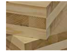
Cross Laminated Timber Manufacturer: Think Wood, Inc 3 Layer CLT Exterior Wall w/ Gypsumboard Insulation CLT panels consist of layered lumber boards (usually three, five, or seven) stacked crosswise at 90-degree angles and glued into place. Finger joints and structural adhesive connect the boards. Board thickness typically varies between 5/8 inch to 2 inches. The panels can be manufactured at custom dimensions, though transportation restrictions dictate their length.
